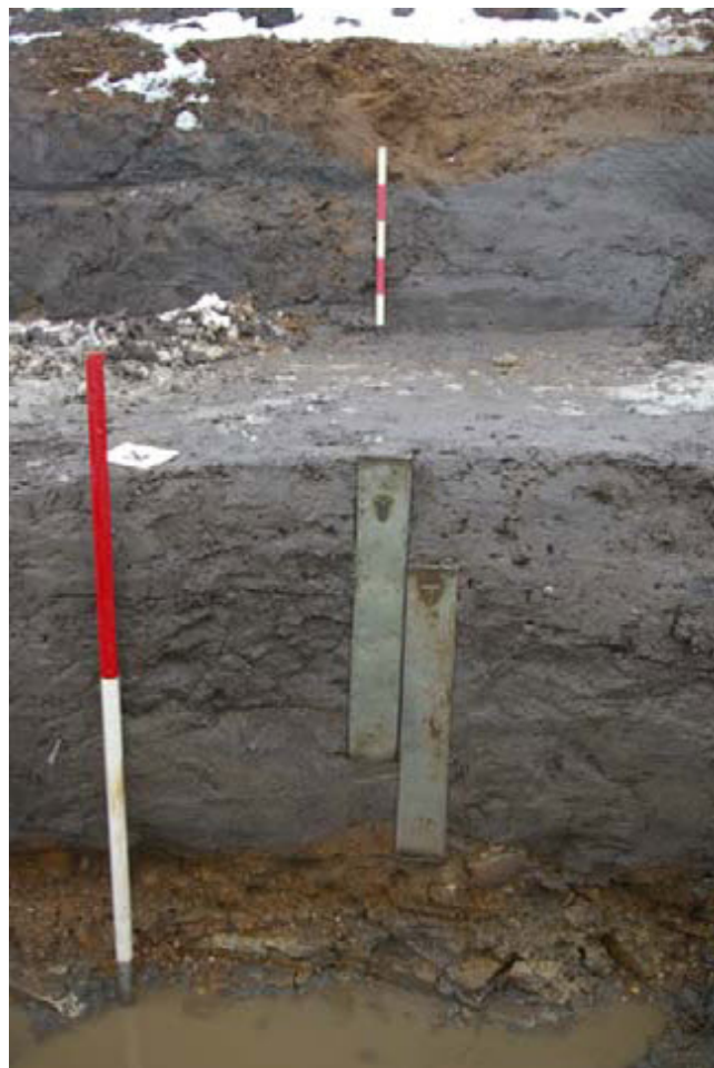
Monolith sampling the silted channel within the Baginton formation. The deposits contain the remains of plants insects and crustaceans.
