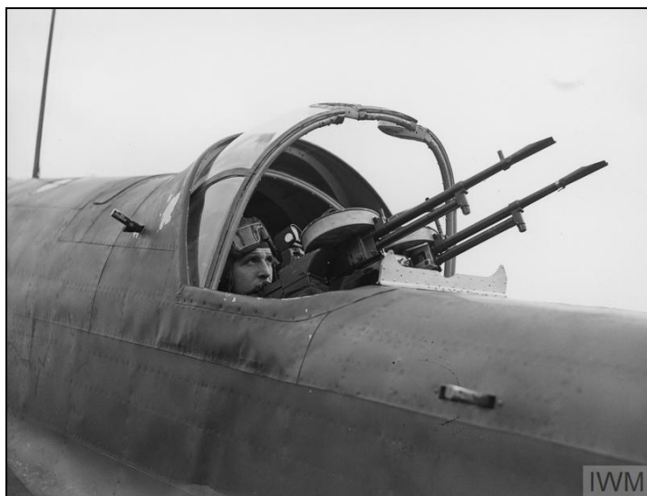
The wireless operator/gunner of a Hampden manning his twin Vickers K guns, 1940. © IWM HU 107827. Reproduced with permission.
